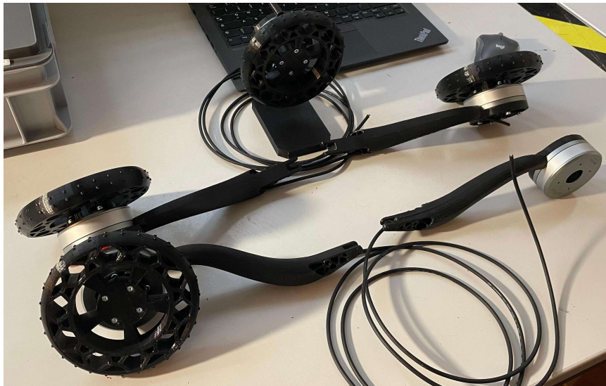
Figure 3.24: Three assembled and one partially-assembled shank, together with the test stand.
