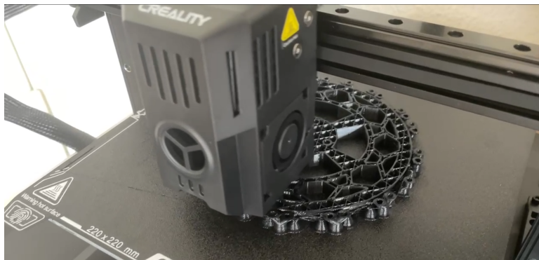
Figure 3.5: Wheel being printed in black TPU.
