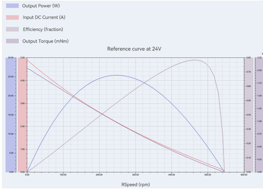
Figure 2.3: Motor Mapping accessed from the T-Motor website [19]
